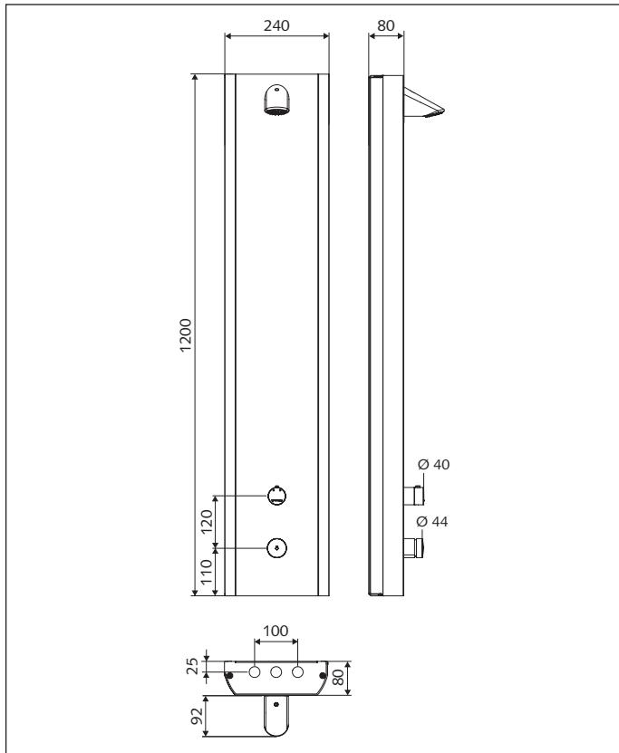
IT Pressione idraulica: 1,0 - 5,0 bar
