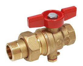
Ball valve, female-tail piece male threaded connections, with probe holder M10x1 mm female threaded, for probe Ø 6 mm. Full port.
