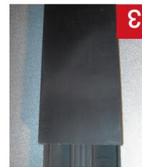
To prevent the hook closure strip opening as the installation procedure progresses, the cover installation strips should be slotted in above the hook closure strip.
