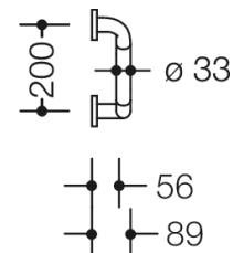
Abmessungen in mm
